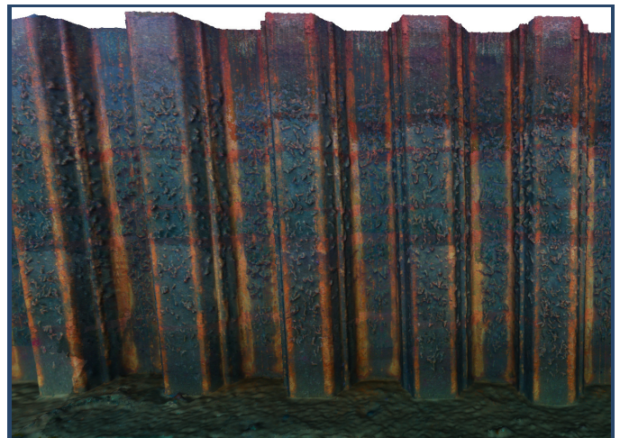
Maps are captured in true colour and tracks surface changes down to the millimetre in accuracy.
